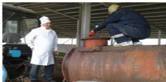
Picture 3 - The disinfection trailed UDP unit is designed for use with wheeled tractors
